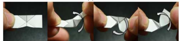
Fig. 4. (a)2D pattern design of Universal joint for SCM (b)Paper Origami trial version of (a). Pitch bending motion (c), Yaw bending motion (d), (e).
